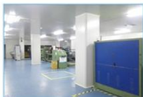
Class 100,000 purification workshop
